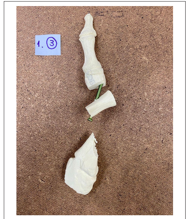
Figure 6. Metatarsal failure. A specimen failure is shown. A fracture line is evident between both screws' entrance.
