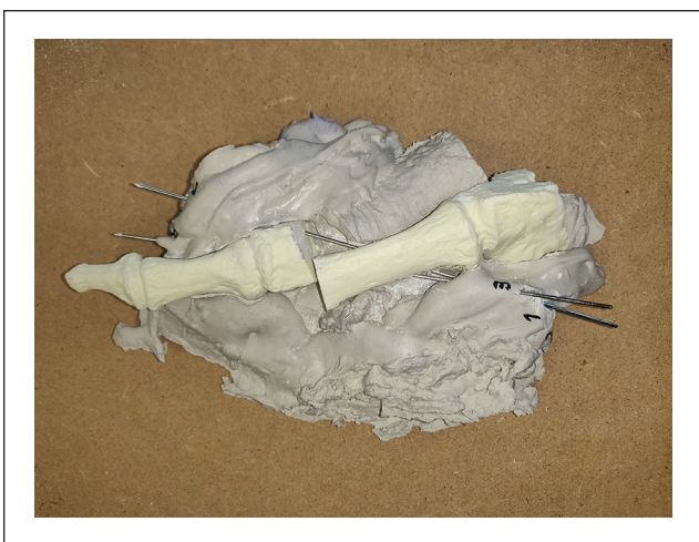
Figure 3. Template. The polymethylmethacrylate (PMMA) first metatarsal osteotomy template is shown here, where bone segments were fixed with a standardized displacement (75%) to avoid variations during the procedure. Using the template, standardized screw-positioning holes were used in order to fix the models in an identical fashion.
