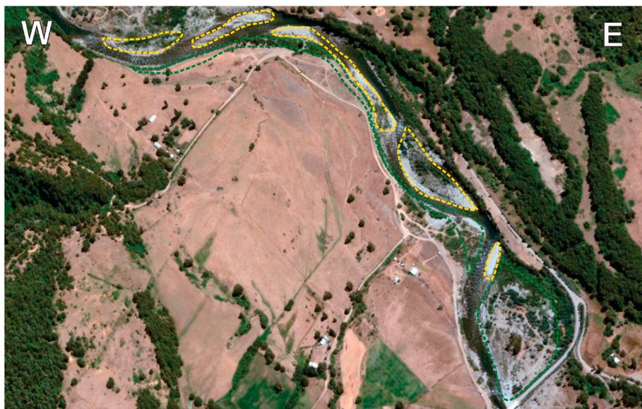
Fig. 13. Satellite view of the Diguillín river in the Atacalco bridge sector. The alluvial plain and the point bar are marked in green and yellow, respectively. (For interpretation of the references to color in this figure legend, the reader is referred to the Web version of this article.)
