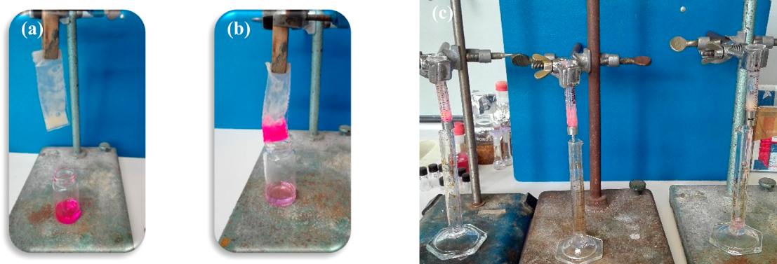
Figure 7. Picture of [\text{C}_{12}\text{C}_{12}\text{im}]_2[2,6\text{-NDC}]/[\text{Bzmim}][\text{NTf}_2] at 5 wt % used in a dialysis membrane (a) before and (b) after 4 h of contact with RhB ( 1.8 \times 10^{-4} M) at 25 °C and (c) sequential system of syringes.
