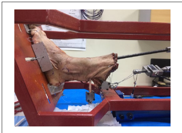
Figure 1. Picture of the special frame designed for the study. The specimen is held against an inclined plane through an endomedullary rod. The actuator pulls the peroneal tendons in line with the tendon excursion.
