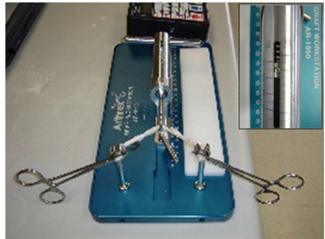
Fig. 2. Tendon tensioning was applied to all samples in group P with a commercially available graft workstation. Insert: Constant tension values applied to all grafts in group P (80 N for 10 min).
